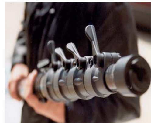
The collapsed 15 metre pole showing the telescopic section locking levers and the locating slot for accepting the grapple hook
