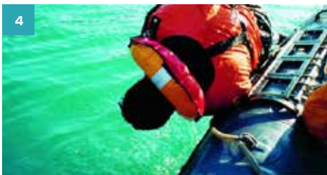
4 The lift takes no longer than 5 seconds due to the cradles 2 to 1 mechanical advantage.
